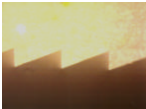
The same view of a fresnel lens molded by Fresnel Optics shows sharp facets and greatly improved replication.
